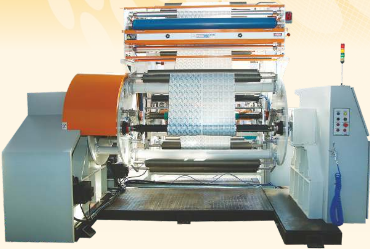
TURRET WITH INTEGRATED SPLICING (Used in converting/offset industry)
